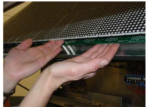
WRONG WAY to lift
