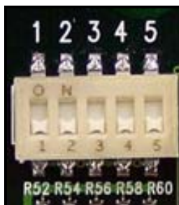
Tune Blaster 1 DIP switch settings: All switches OFF
