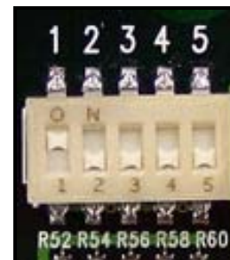
Tune Blaster 2 DIP switch settings: Only switch 1 is ON
