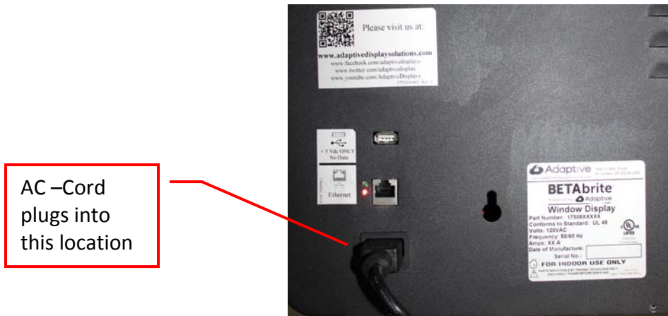
Figure 2: Typical layout of labels and connectors (as viewed from back of sign).
