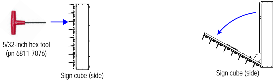
Figure 11: Use a hex tool to open the sign door
