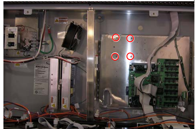
Location of tie wrap holders on a sign with a 12-channel daughter card.
